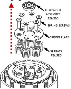
**7.** Using a 17mm socket, remove the center hub bolt. Then, lift the core of the clutch out by gripping the spring posts and pulling upward.
