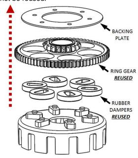
**12.** Clean the rubber dampers and ring gear of all grit and rivet chips leftover from drilling.
