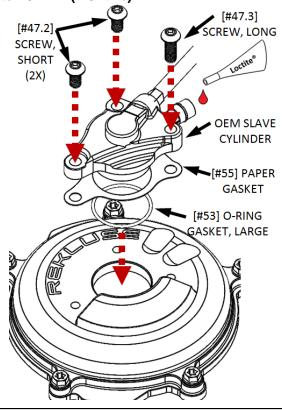
**NOTE:** The long screw [#47.3] **MUST** be placed in the hole location where the slave cylinder housing is thickest (rightmost side of the slave cylinder).
