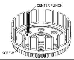
**WARNING**: It is *critical* that you apply Loctite and stake the ends of the screws or they can back out. Rekluse is not responsible for engine damage that may be caused by screws that back out.
