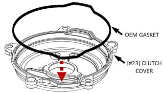
It may be helpful to apply a thin film of clean grease to the gasket to hold it in place in the groove.
