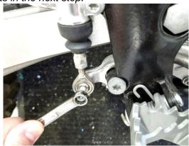
**4.** Remove the slave cylinder from the clutch cover and move it aside, but do not remove the hydraulic line from it.
