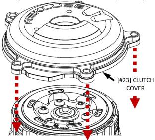
**NOTE:** The *OEM* clutch cover is **not** compatible with any Rekluse clutch product (CoreEXP or CoreManual) because it does not provide adequate clearance to the moving parts. The Rekluse clutch cover **must** be used with any Rekluse clutch product.
