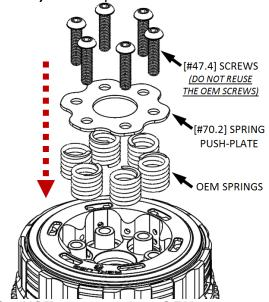
DO NOT reuse the OEM screws, as interference with the clutch cover will occur.
